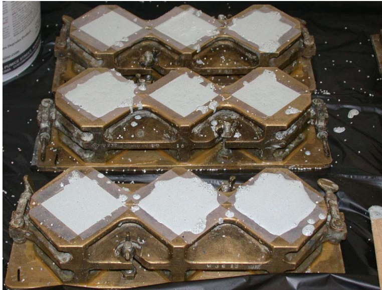
Figure 1. Cube specimen fabrication
