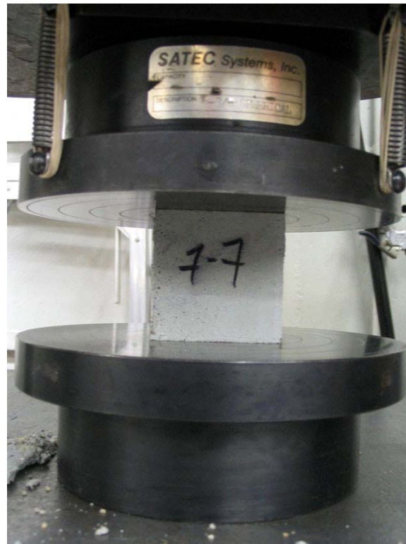
Figure 2. Compressive strength testing
