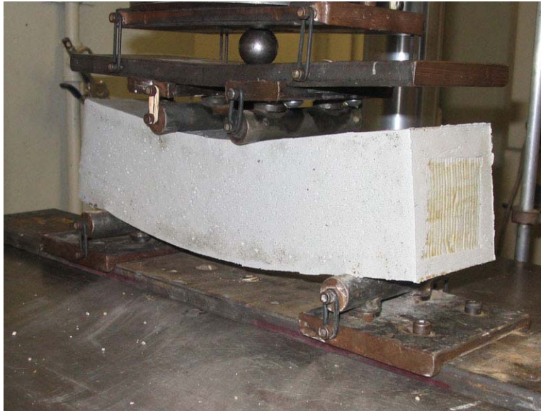
Figure 3. Flexural strength testing
