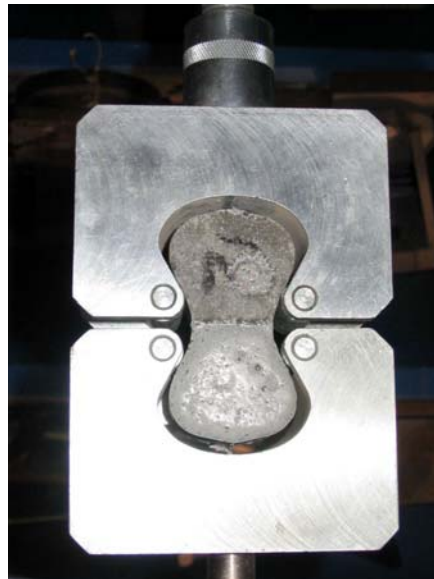
Figure 2. Dog-bond specimen for bond testing.
