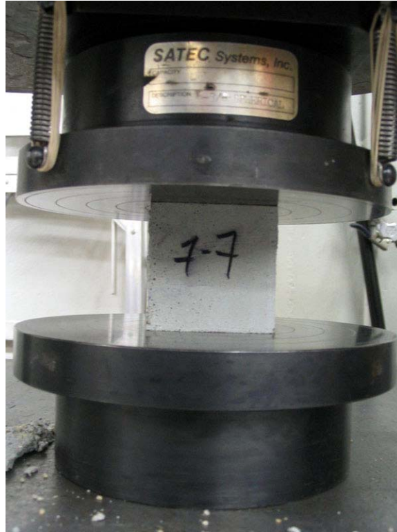
Figure 3. Compressive strength testing
